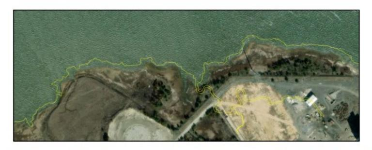
Figure 3. NJ Tidelands Claim Line showing >35feet of tidal wetland loss from 2002-2023, or ~0.8ft/yr.
